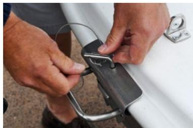
Left: Locking the bow with the stainless steel bolt
