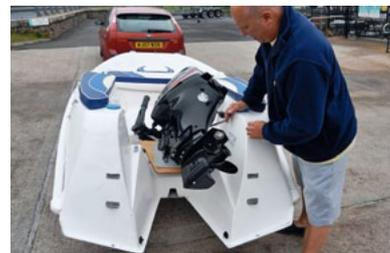
Right: The engine folds up into the aft end of the cockpit
