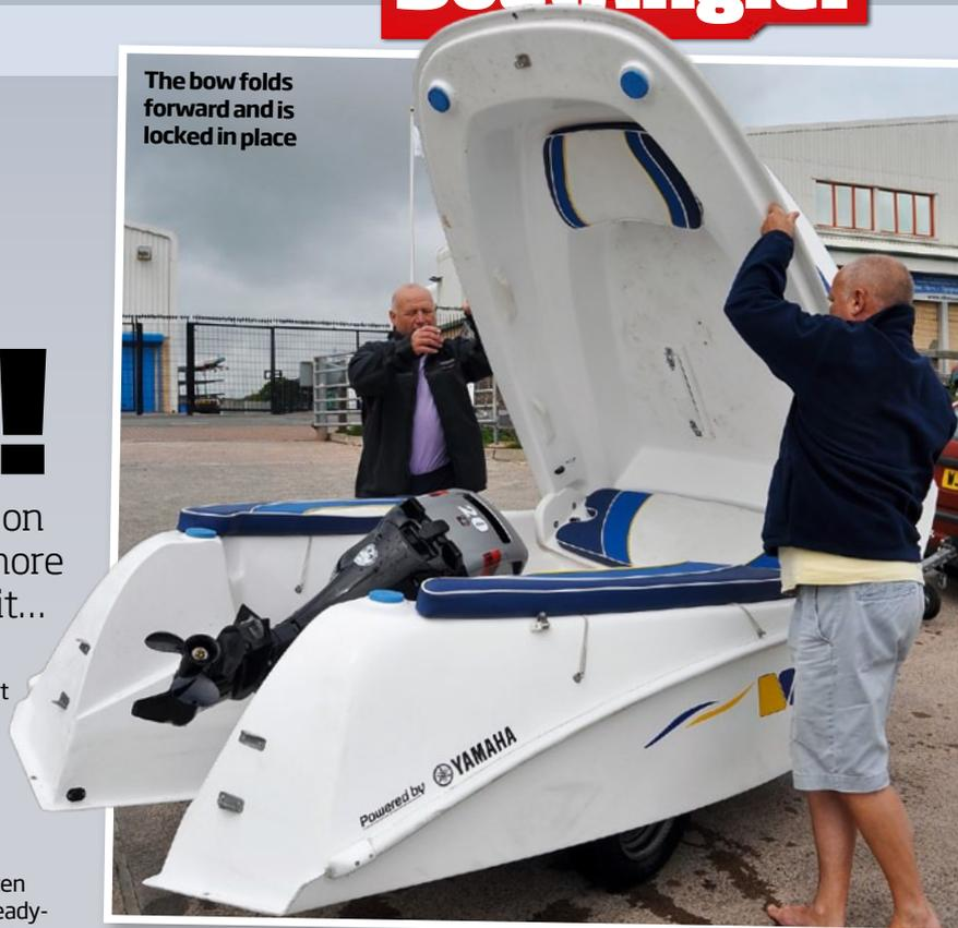
The boat has tiller steering and takes an outboard engine up to 25hp
