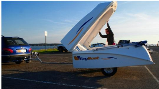
With the EzyBoat there is no need to separate the trailer from the boat. The wheels can be retracted into the boat with a simple push of a lever once the craft is afloat. What’s more, the EzyBoat folds in half, making it very easy to tow behind any size car and easy to store in a garage or parking space.
